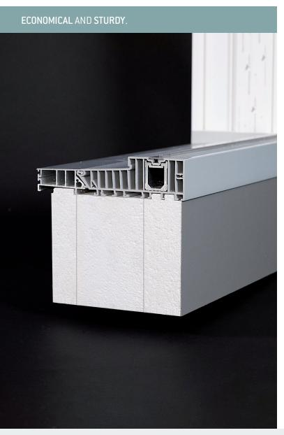
The Lift & slide support packer is a combination of two external structural support layers with a light, non-structural, insulating core. This combination reduces the overall weight of the packer, provides excellent thermal performance and the clever combination provides a cost saving. The two external structural sections provide adequate support for the lift and slide door system and also allow the packer to be easily and securely fixed to the building substrate and the threshold profiles.
