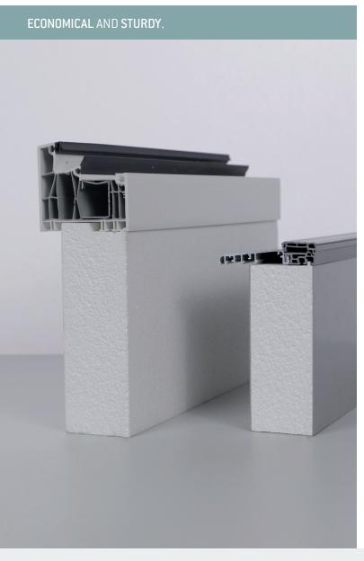
The CF support packer is a combination of strength with excellent thermal insulation and very low weight. The material provides excellent thermal performance adequate support for the threshold and also allows the packer to be easily and securely fixed to the building substrate and the threshold profiles. Thanks to the stable, waterproof construction material, attachment from all sides are possible.
